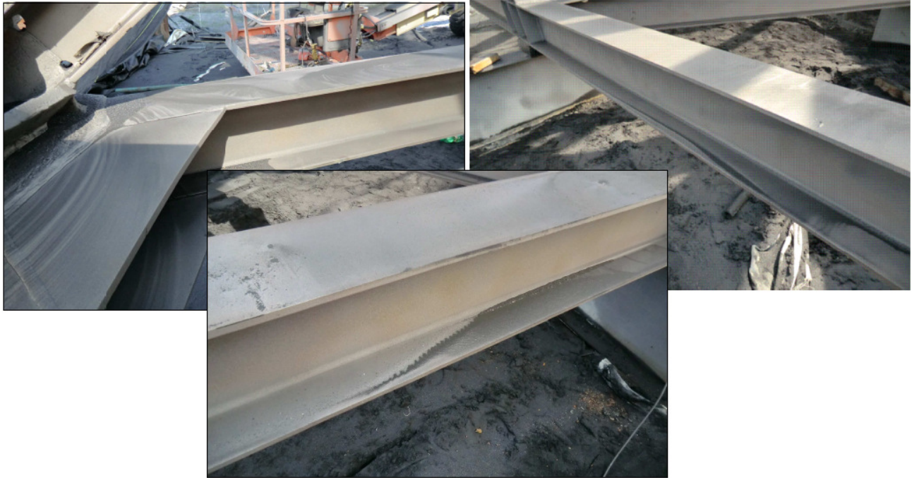
Figure 6: During resonance, patterns of high and low amplitude become apparent, even visible, on the work-piece. During the treatment of the 3 rd work-piece, which was done not long after it had been shot-peened, these patterns become evident, as shot-peened that had been resting on the work-piece was driven off the high-amplitude locales, and came to rest on low-amplitude locales. Such patterns define the nodes of the work-piece, and are referred to as a nodal pattern . Different resonant peaks generate different nodal patterns, indicating that the effect of the vibrator is relocated, not by moving the vibrator, but by tuning the vibrator to different resonance frequencies, which generate a different nodal pattern.
