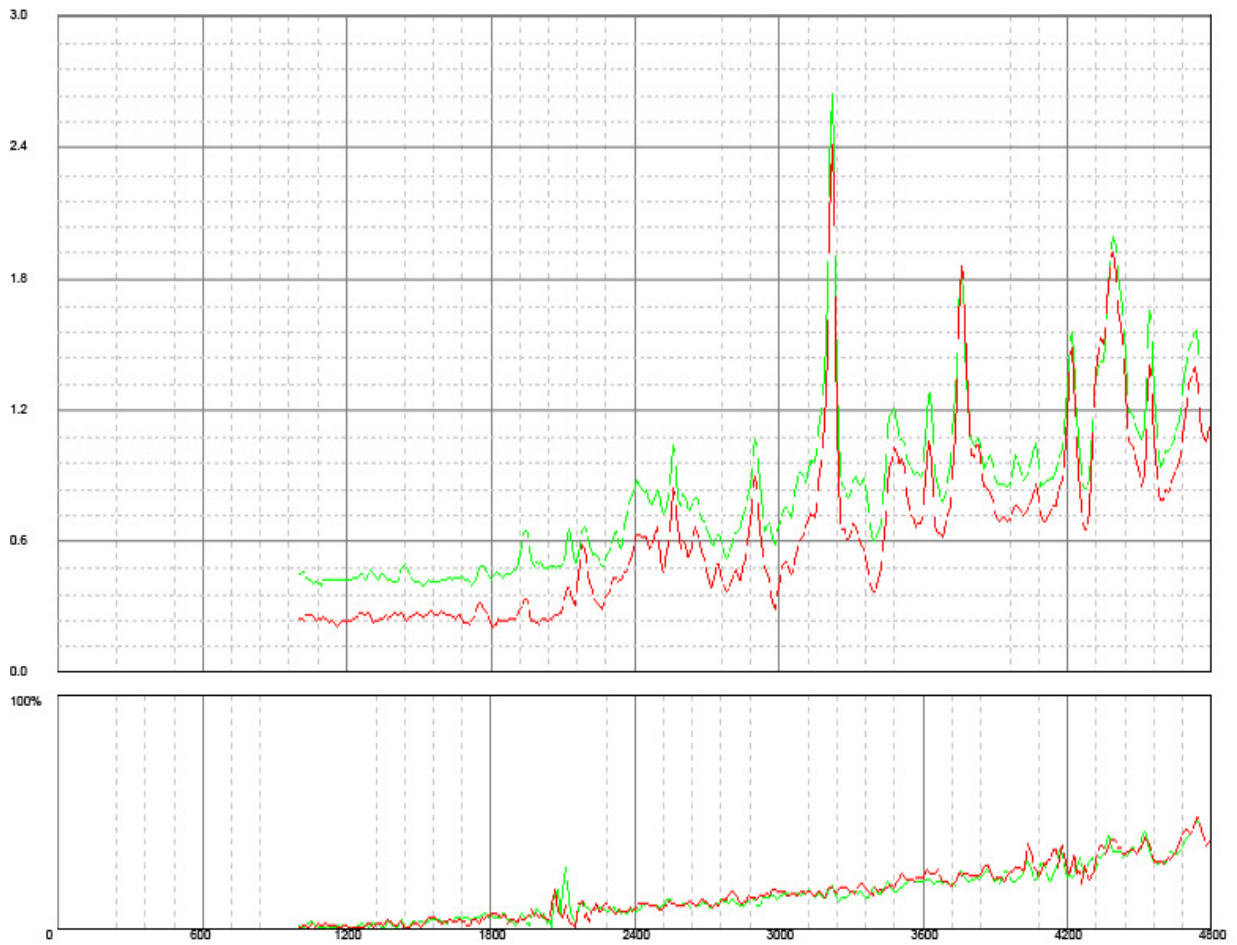
Figure 12: Work-piece 3, 2 nd treatment. Changes in resonance pattern were subtle, indicating that the first treatment was successful in stabilizing the workpiece.
