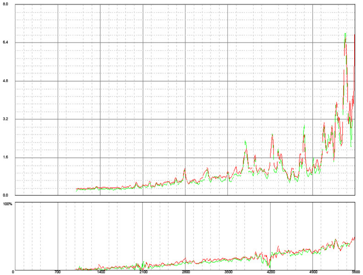
Figure 13: Work-piece 4, 1 st treatment. Max RPM = 5600, vibrator unbalance = 35%. The last workpiece showed only subtle changes during VSR Treatment, both during the 1 st and 2 nd treatments.
