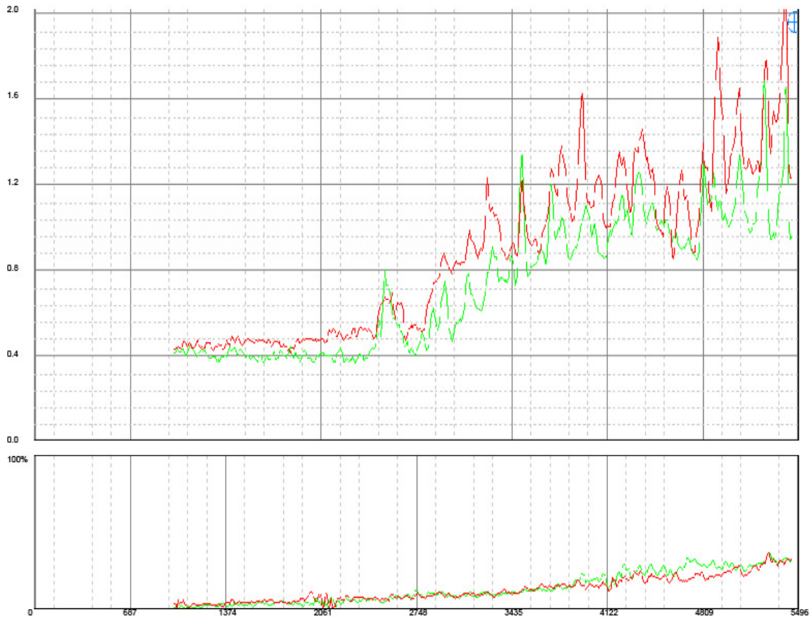
Figure 9: Work-piece 2, 1 st treatment, max RPM 5500, vibrator unbalance 35%. Larger peak growth (as compared to the 1 st workpiece) can be seen during this treatment, esp. above 4800 RPM.
