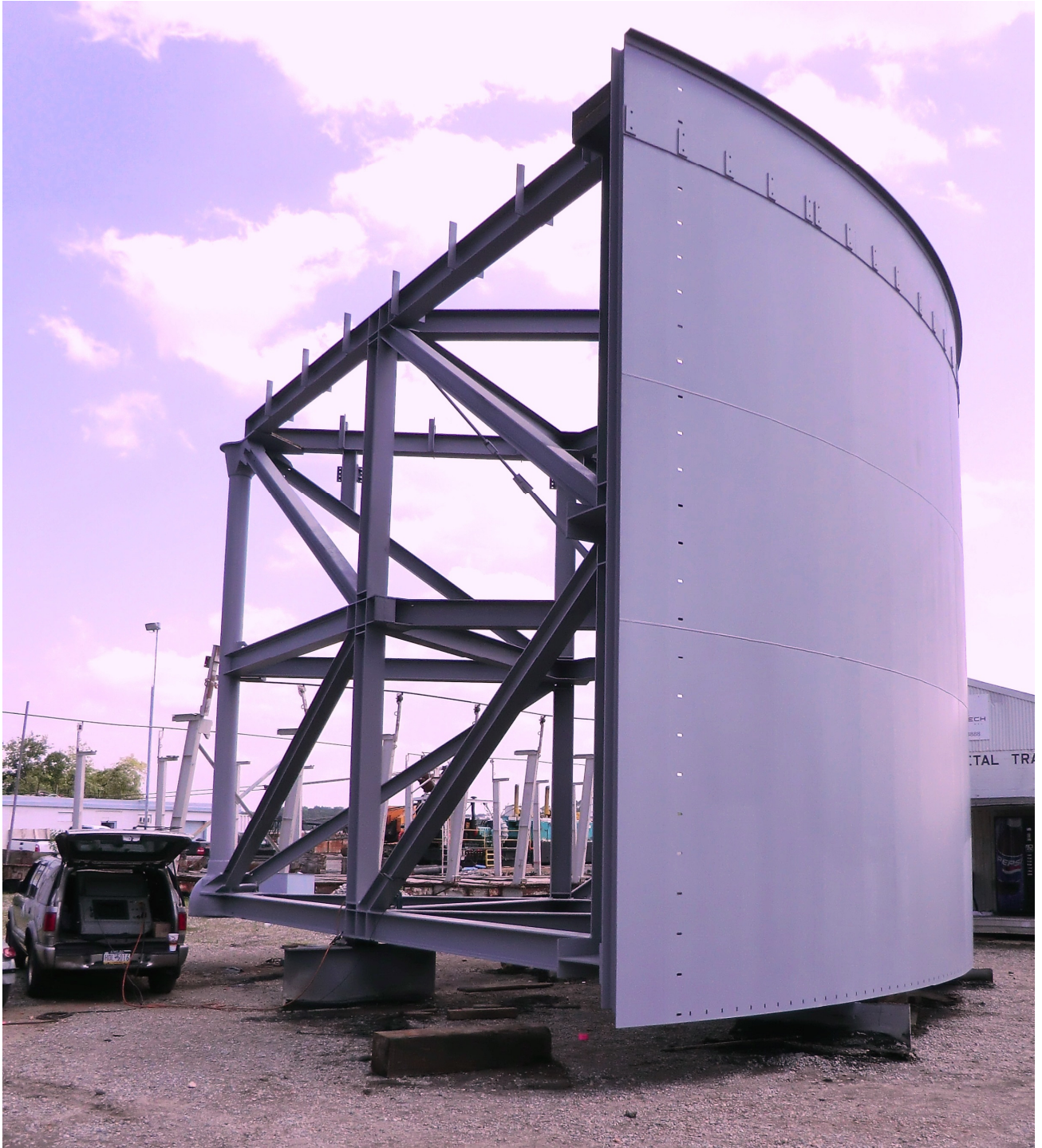
Figure 3: VSR Setup. The work-piece was placed on 4 load cushions (measuring 1' X 1' X 4" H), two of which were very close together, effectively functioning as one cushion.
